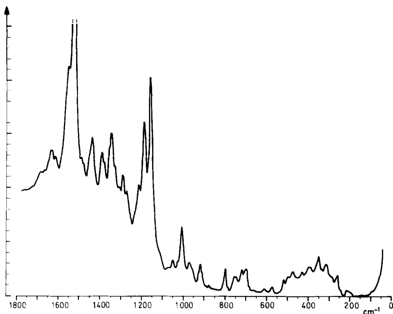
Figure 1. Resonance Raman spectrum of spinach chloroplasts under 4416 Å excitation. The chlorophyll a contribution is preponderant over that of chlorophyll b. Bands from carotenoids arise at 965, 1005, 1160, 1190 and 1527 \text{cm}^{-1} . Resolution at 1000 \text{cm}^{-1} : 8 \text{cm}^{-1}
